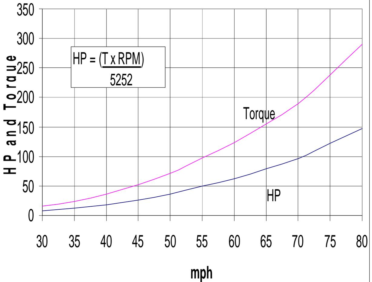
The energy needed to push air out of the way is termed aerodynamic drag. General Motors published test data on how much horsepower (HP) it takes for a standard 26' GMC to drive at different speeds.
