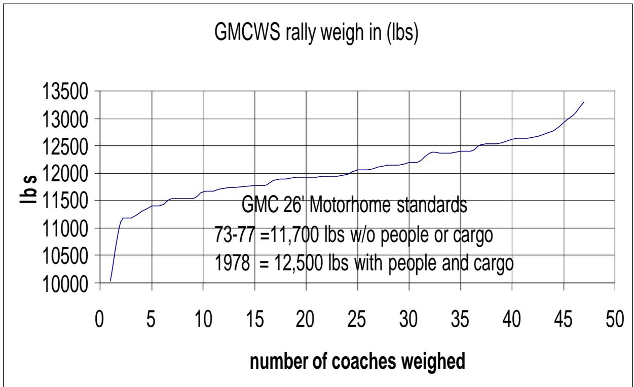
This “weigh in” was done in conjunction with the GMCWS Tire Safety Seminar and it shows that nearly half of the coaches were overweight compared to the GMC Design and testing standards. This “weigh in” did not include tow weights. Coaches and tows in combination that weigh more than the specifications and drive slower than the 75 mph design criteria are candidates for increasing the final drive gear ratio.
