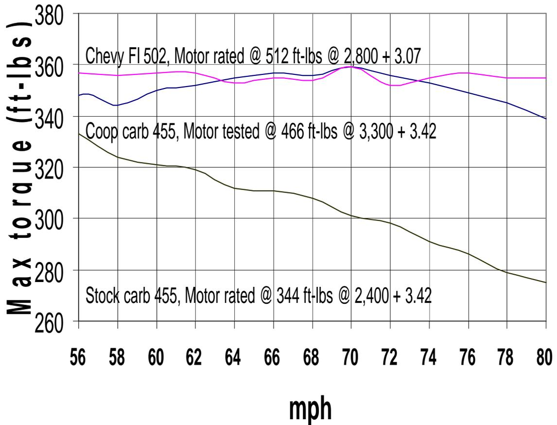
This chart shows the difference between the best stock GMC dyno tested (Cerrina) with 3.42 differential gear ratio and the dyno tuned Coop-motor with the same differential gear ratio. For comparison, I also plotted a Dyno tuned GMC with a Fuel Inject 502 Chevy motor with a stock 3.07:1 differential gear. It shows that the 455coop motor with 3.42:1 gearing is very close to the same maximum torque produced by the larger FI 502 Chevy motor with the stock 3.07 gearing.
