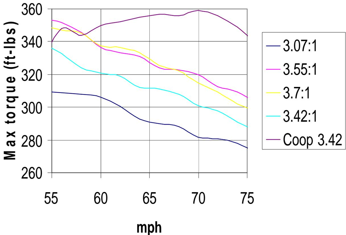
I took the dyno test data of the best stock 454 (Cerrina rebuilt motor with 3.42 differential) and extrapolated that data by changing the speed and torque at that speed to what it would be with the most common listed differential gear ratios. The calculated results shows the effect of that rapidly decreasing motor torque with increasing rpms with the cross over the 3.55:1 and 3.7:1 happening at around 67 mph.
