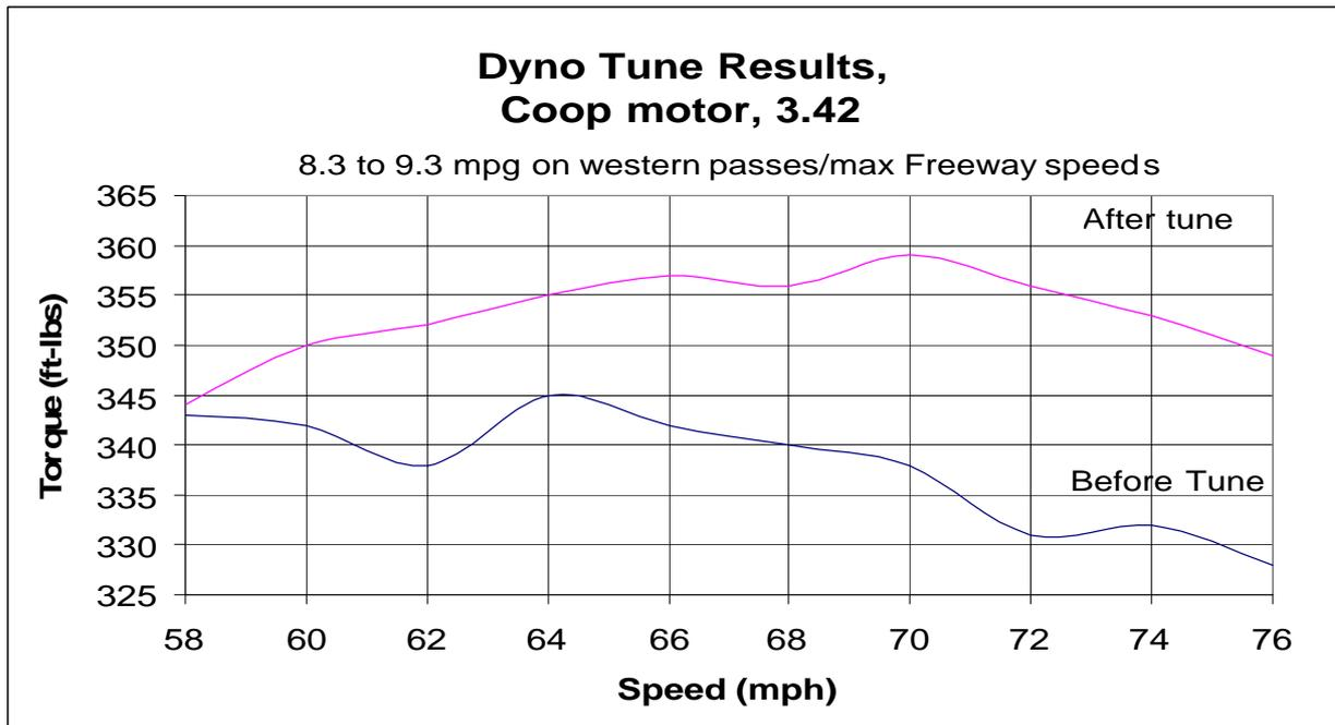
The change in maximum torque tuning shows how the increased A/F ratio increased the available torque at 70 mph by 20 ft-lbs or an additional ~6% while also producing a one mpg improvement while cruising at freeway speed limits.
