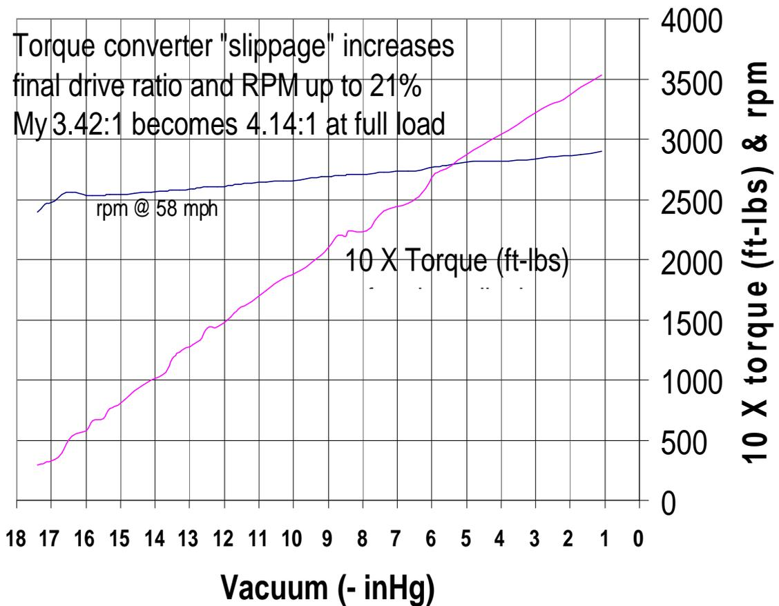
This is unique to the GMC Motorhome Turbo Hydro-Matic Transmission. It shows how an increasing load at a constant speed increases the vacuum, torque, and rpm by continuously changing the effective gear ratio by what we hear as Torque converter "slippage". Under maximum torque conditions, the 3.42:1 differential gearing effectively becomes 4.14:1 gearing. To show these interrelationships, I chose to multiple the torque values by ten so that it would have the same Y scale as rpm.
